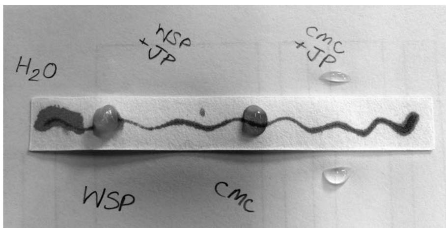
Figure 10, Experiments showing the degree of ion migration incurred from a line of iron gall ink drawn on Iron (II) Ion indicator paper when exposed to (left to right) water; wheat starch paste; wheat starch paste in a Japanese paper enclosure; Sodium CMC Carboxymethyl Cellulose (SCMC); Sodium CMC Carboxymethyl Cellulose (SCMC)in a Japanese paper enclosure; and rigid Agar gel.
